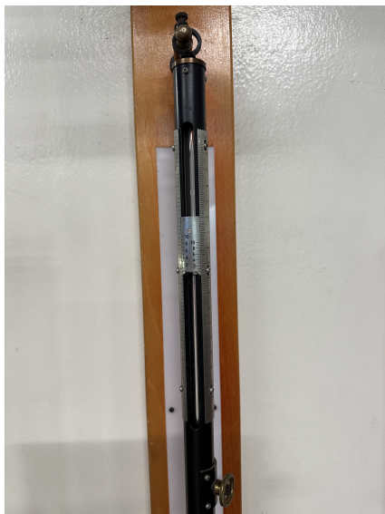
Fig. 1 Barometer used for measuring atmospheric pressure.
