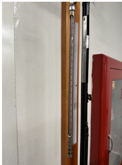
Fig. 2 Thermometer used for measuring room temperature.
