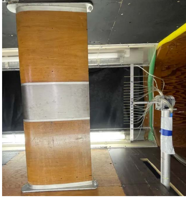
Fig. 6 Airfoil mounted vertically in test section with wake rake behind trailing edge.
