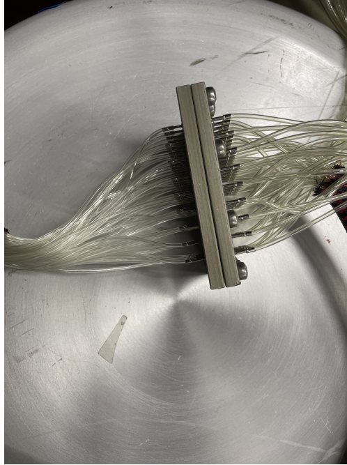
Fig. 4 ScaniValve hardware tube connection.
