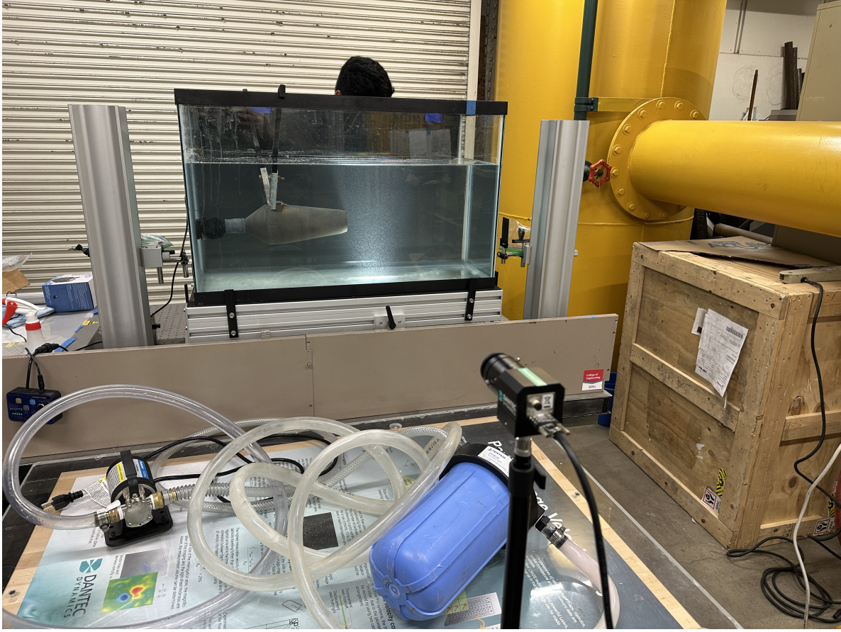
Fig. 3 Full experimental setup showing the water tank, camera, optics, and pump system.
